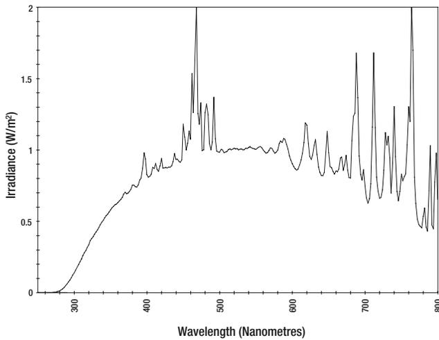
Figure 7: Spectroradiometer irradiance measurement of a Xenon arc lamp
