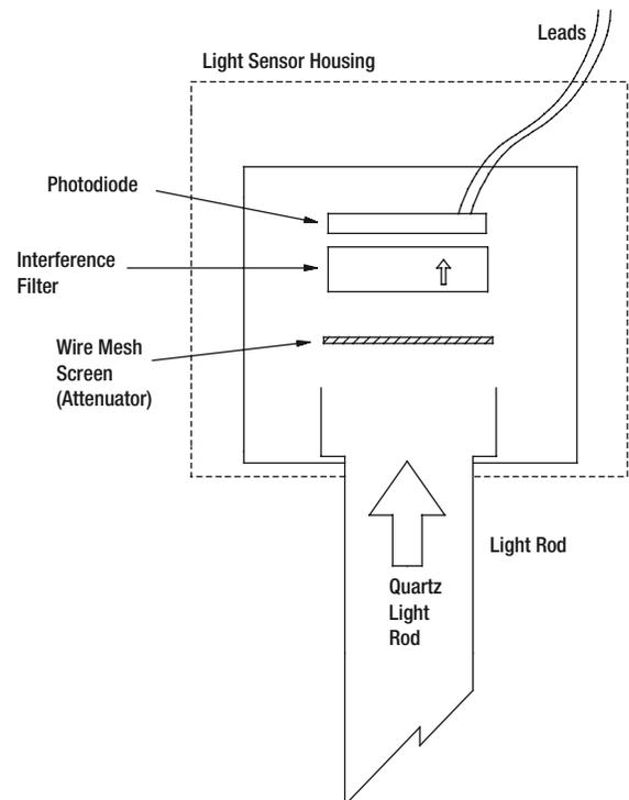
Figure 12: Light monitor sensor housing
