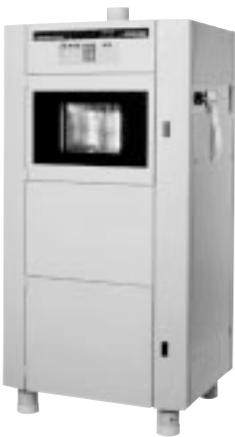
*Atlas laboratories offer the most accelerated, up-to-date testing, including in our air-cooled Xenotest Alpha.*
