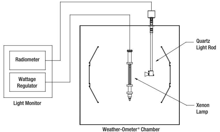
Figure 11: Controlled irradiance system
