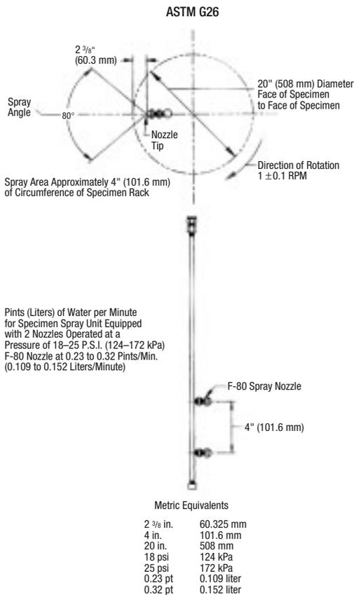
Specimen Spray Arrangement for Type A and AH Apparatus
