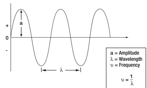
Figure 3: Properties of a wave
