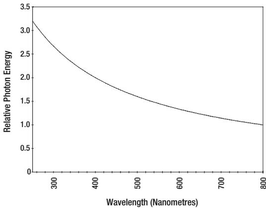
Figure 4: Relative photon energy as a function of wavelength
