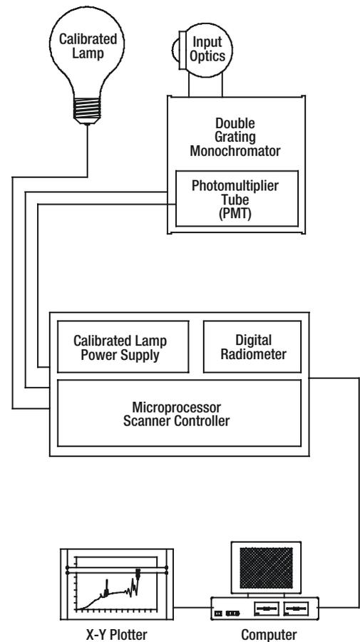
Figure 8: Spectroradiometer system block diagram
