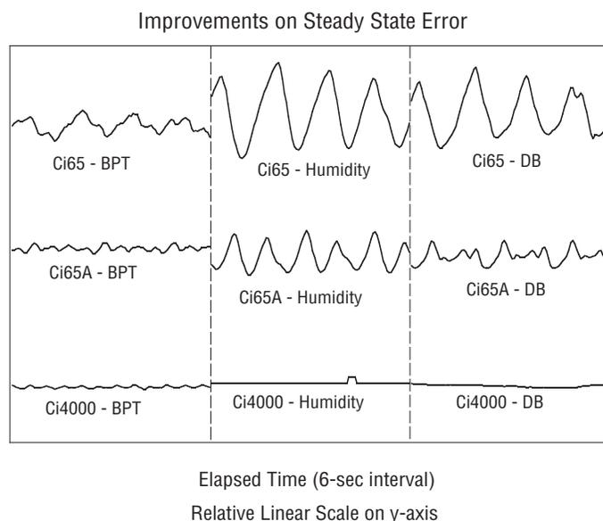
*Figure 4: Actual tolerance of black panel temperature (BPT), relative humidity (RH), and chamber air temperature (CHT = DB) through three generations of weathering instruments*
