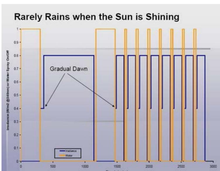
Test sequence according to ASTM D7869 - An improved accelerated weathering protocol to anticipate florida exposure behavior of coatings\*
