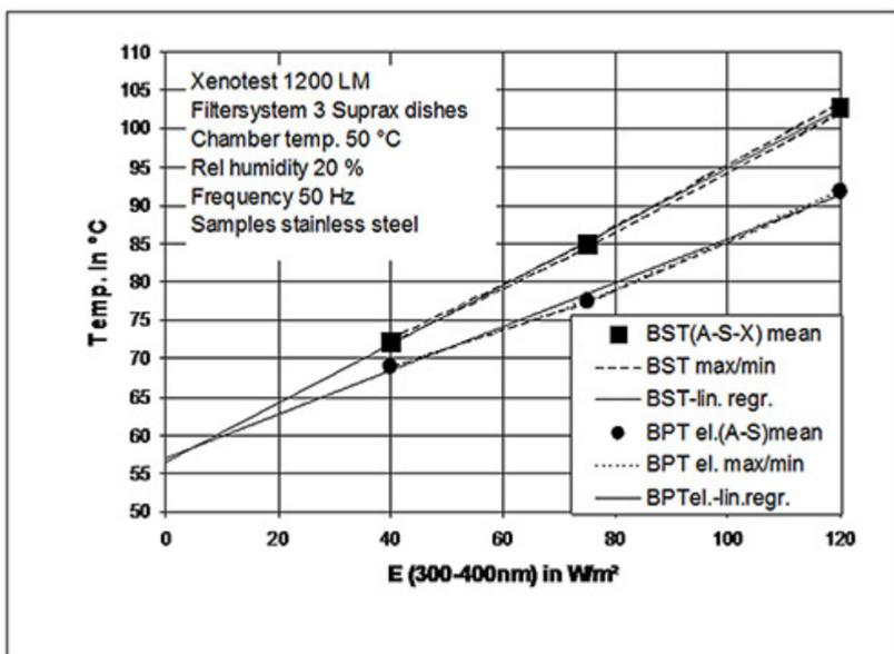
Fig. 1. BPT and BST in dependency of the irradiance in an Atlas Xenotest® instrument
